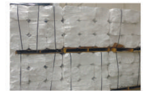
after cold compacting
